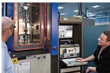
LAB TESTING A MAGNERIDE DAMPER AT BWI'S TCP
