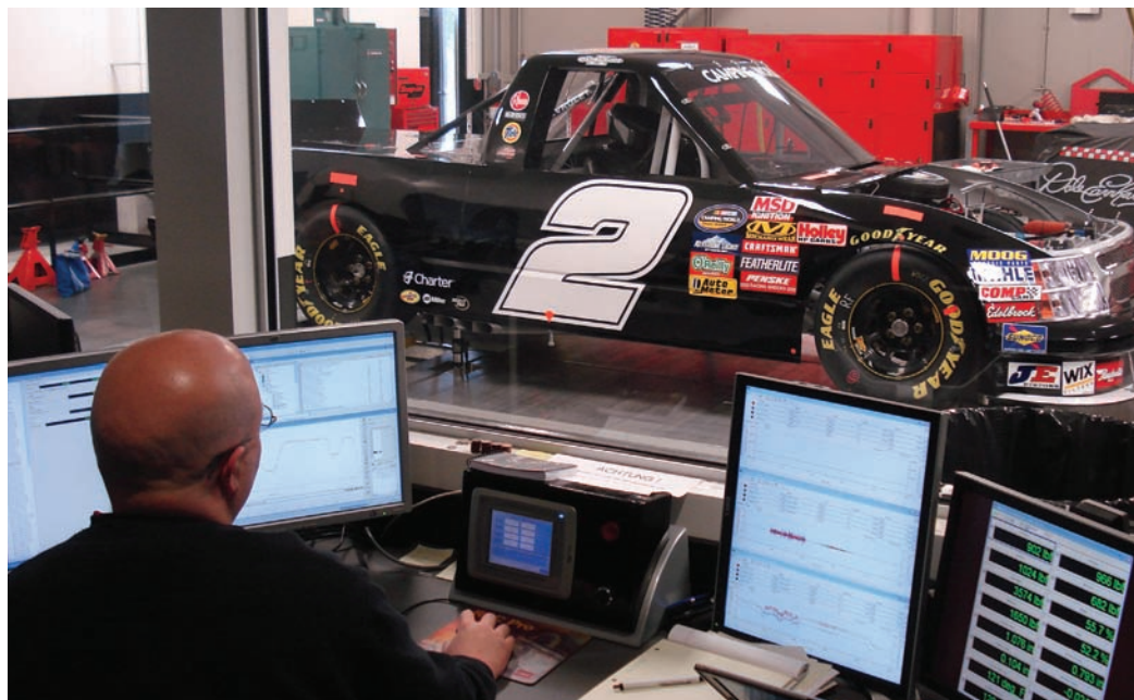
ABOVE: DR KEVIN KEFAUVER PREPARES TO LAUNCH A TRACK SIMULATION ON EARNHARDT TECHNOLOGIES' SEVEN-POST RIG IN MOORESVILLE, NORTH CAROLINA, USA. AMERICAN STOCK CARS, SUCH AS THIS CAMPING WORLD TRUCK SERIES CHEVROLET, HAVE UNIQUE AERODYNAMIC CHARACTERISTICS THAT DEMAND CAREFULLY DEVELOPED SETUPS – WITH SPECIAL ATTENTION TO BODY CONTROL METRICS
