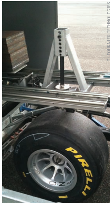
ABOVE: ELEGANT AND PORTABLE TIRE TESTING SKID TRAILER DESIGNED BY DUFOURNIER TECHNOLOGIES TO CAPTURE TIRE/SURFACE INTERACTIONS AT VARIOUS PROVING GROUNDS AND RACETRACKS
