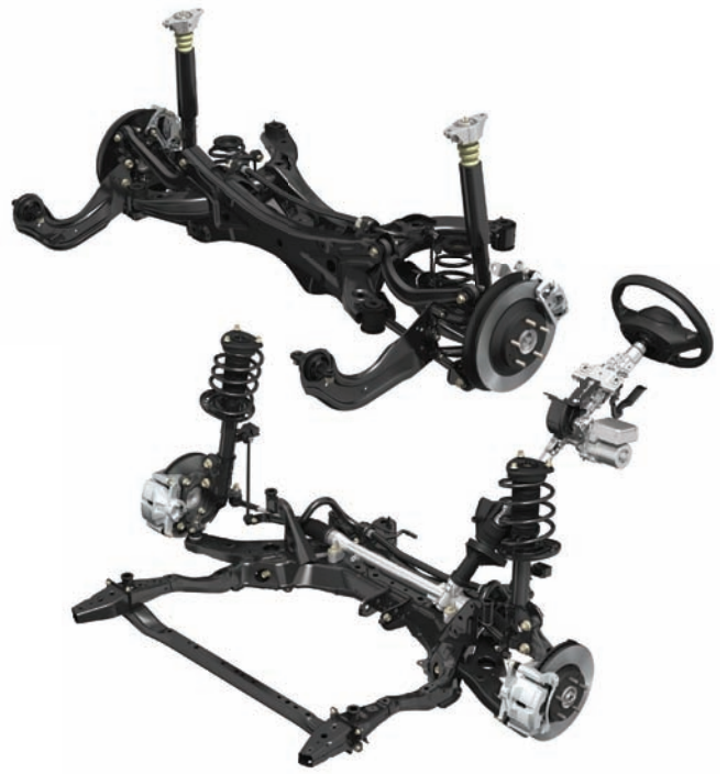
CX-5 FRONT AND REAR AXLES. THE SUBFRAME AND CROSS MEMBERS HAVE BEEN EXTENSIVELY REWORKED
