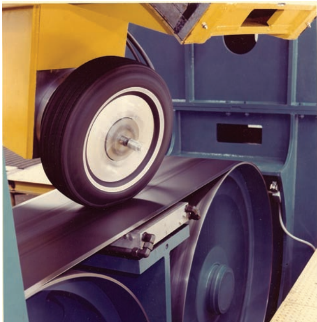
CALSPAN'S TIRF OPENED IN 1973. THIS IS THE ORIGINAL FLAT ROADWAY TIRE TEST SYSTEM
