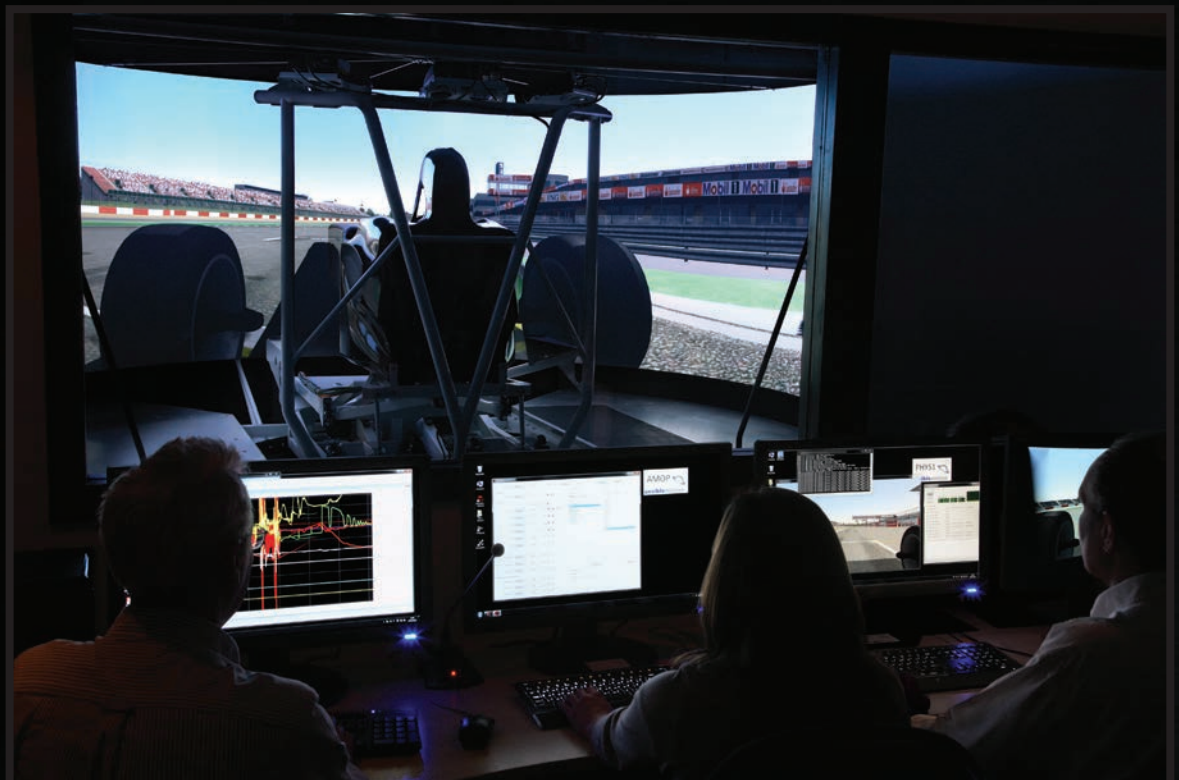
MAIN: AN H2IL SIMULATOR USING ANSIBLE MOTION'S 6DOF PLATFORM, HANDWHEEL LOADER, DYNAMIC VISION SYSTEM, AND CUEING STRATEGIES
