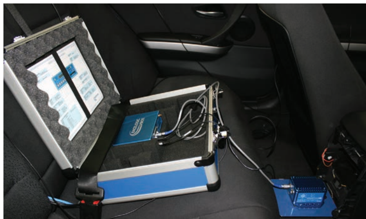
LEFT: 100HZ VBOX3I AND IMU PROVIDE A STABLE BASE FOR THE ABD SR60 STEERING ROBOT
