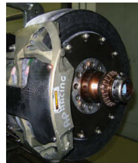
INSET: REAR SPRING-DAMPER SETUP FEATURING DSSV DAMPERS AND EIBACH SPRINGS. PUSHROD CONFIGURATION IS EASY TO WORK ON ABOVE: FRONT BRAKE DETAIL SHOWS FLOATING CARBON-FIBER DISC WITH AP RADI-CAL SIX-PISTON CALIPERS
