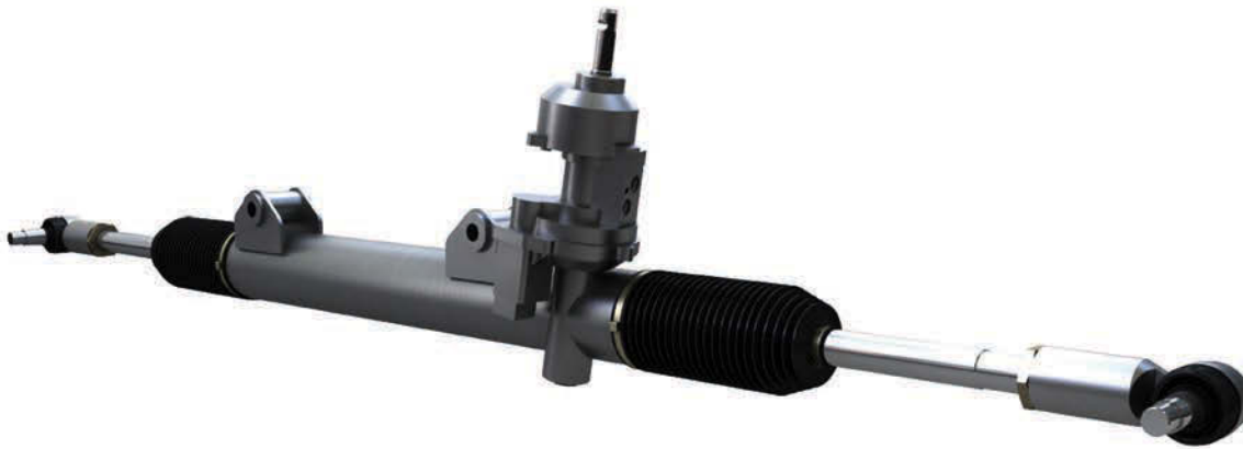
TOP: THE OPTIONAL USE OF IHSA TECHNOLOGY AS AN ADD-ON MODULE IN HYDRAULIC RACK-AND-PINION STEERING FACILITATES THE INCORPORATION OF ALL SAFETY AND COMFORT FUNCTIONS IN THE HEAVY VEHICLE CLASSES FOR THE FIRST TIME
