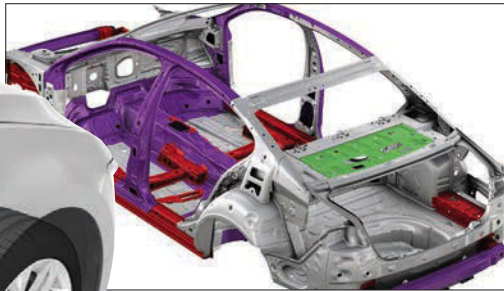
ABOVE: THE CUTAWAY SHOWS THE DISTRIBUTION OF METALS WITH VARIOUS GRADES AND STRENGTHS WITHIN THE PASSAT'S SHELL
