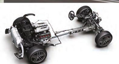
wheels with no fixed distribution, with up to 100% of the torque being diverted to either wheel at any time. The first-generation car's viscous central coupling has been replaced with another multiplate clutch arrangement, while the rear differential remains a purely mechanical locking unit, which allows for 25% locking effect in traction, and 45% in thrust.
