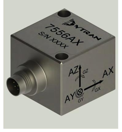
ABOVE: THE MODEL 7556A2 IS A FULLY ANALOG SIX DEGREE OF FREEDOM (6DOF) SENSOR CONTAINING A MEMS-BASED TRIAXIAL ACCELEROMETER AS WELL AS THREE MEMS-BASED GYROS
