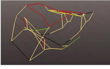
ABOVE: BODY STRAIN MEASUREMENTS LEFT: BODY DEFORMATION DURING MANEUVERS
