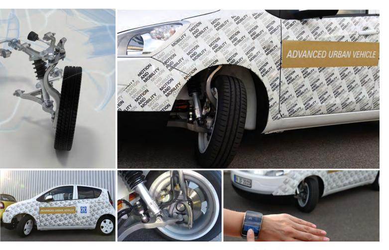
Naunheimer. "We could do 50km/h with the tires angled at 75°, but the risk of instability is greatly increased, so we have made some limitations to the steering system so that the angle halves at speed."
