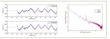
FIGURE 4: MEASURED ROAD PROFILE AND POWER SPECTRAL DENSITIES ON LEFT AND RIGHT SIDE OF VEHICLE
