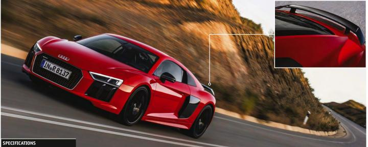
Audi R8 V10 (V10 plus) Dimensions: 4,426mm (L) x 2,037mm (W inc. mirrors) x 1,240mm (H). Wheelbase: 2,650mm. Track width: 1,638mm (F), 1,599mm (R) Dry weight: 1,454kg Powertrain: 5,204cc V10. 540PS @ 8,250rpm (610PS @ 8,250rpm), 540Nm @ 6,500rpm (560Nm @ 6,500rpm)
