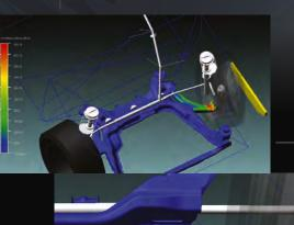
Large deformation of lower control arm during a curb strike
