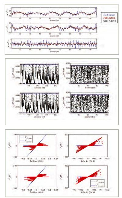
and minimum constrained forces on the lower dampers. It is also evident that unsprung mass experiences more vertical deflection velocity than sprung mass, and thus more vibrations are dampened by the lower damper. The saturation limit on the upper damper is greater than that of the lower damper, which is also evident from the slope of  $F_{low,min}$  being greater than the  $F_{Low,max}$ .
