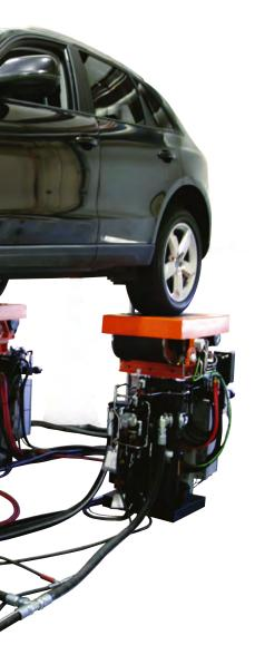
and repeatable means of performing directly observable full-vehicle vibration analysis, benchmarking, suspension tuning and validation. Engineered to deliver high-fidelity ride comfort simulation, it enables fast and efficient acquisition of meaningful component, subsystem and full-vehicle performance data earlier in the development cycle. In other words, engineers can run more iterations in the lab, reserving the test track for final validation.
