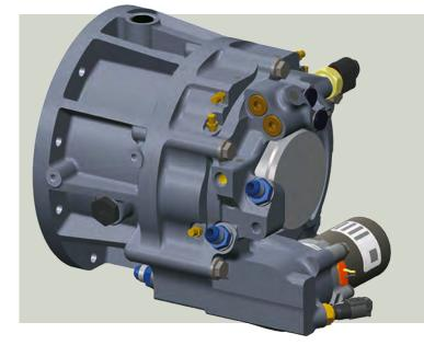
between the 19-tooth wheel and the 21-tooth wheel by applying a clamping force to a small wet clutch located at the end of each planet shaft. If no clamping force is applied, the cTV is inactive and the rear drive unit works in the traditional manner. The clutch clamping force is obtained via annular hydraulic pistons located on each clutch.
