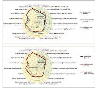
(typically 'comfort', 'neutral/normal', and 'sport') to calculate the best damper settings in each situation in real time via electrical current sent to the electronic valves.
