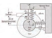
FIGURE 2: FULL ACTIVE CONTROLLER AND DOUBLE DAMPER-BASED SEMI-ACTIVE CONTROLLER AT FRONT LEFT SIDE OF VEHICLE
