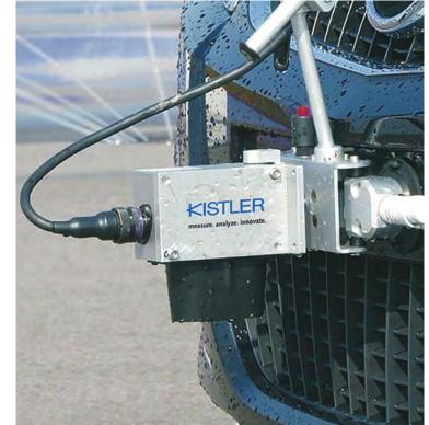
decelerations. For future evaluation, it is necessary to determine the rise time of the brake pressure.
