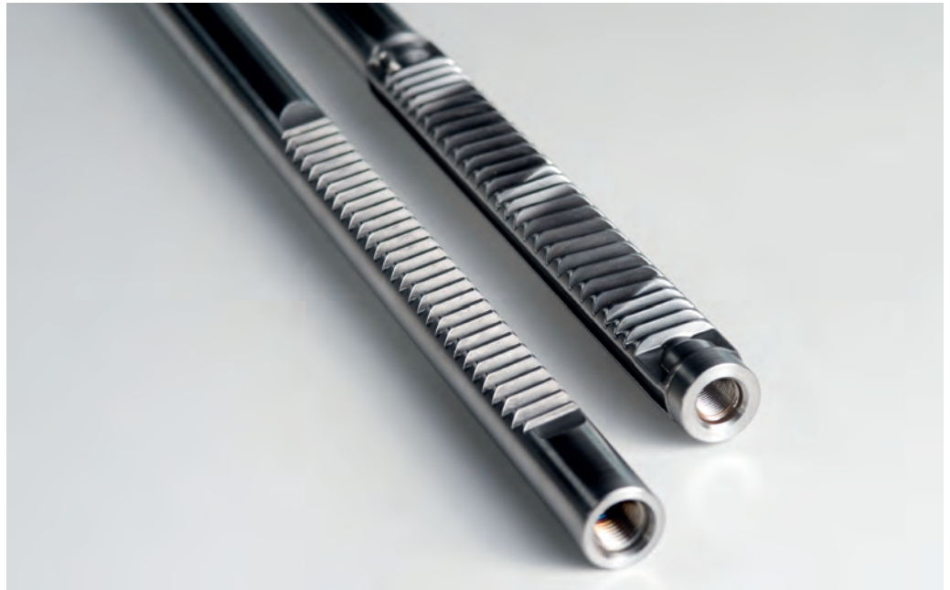
ABOVE: Precision warm-forged rack bars (the bar on the right) have forged teeth, enabling a wider, deeper cross section
