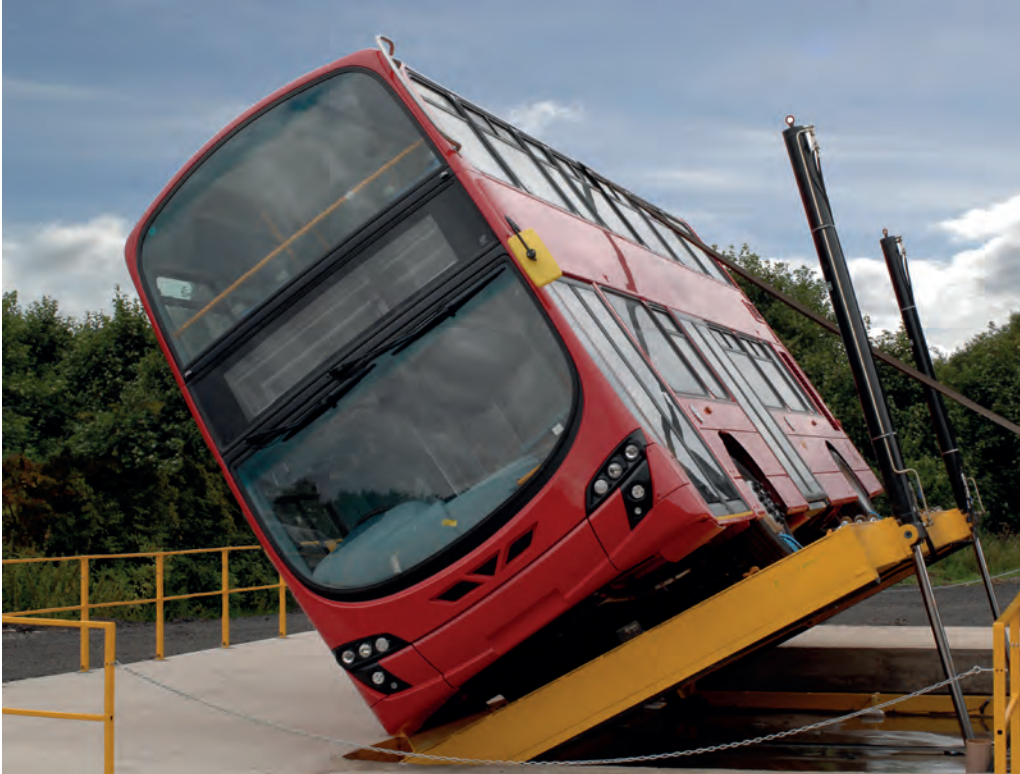
ABOVE: Millbrook's 9m x 3.3m tilt platform can tilt vehicles weighing up to 42,000kg at an angle of up to 45°
