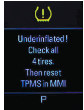
THE 2009MY AUDI A6/S6 IS THE FIRST MODEL ON THE US MARKET WHICH HAS AN INDIRECT TPMS CONFORMING TO FMVSS 138
