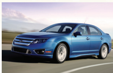
VEHICLES OF DIFFERENT SIZES, HEIGHTS AND WEIGHTS SHARE THE CD3 PLATFORM FIRST USED ON THE MAZDA6 FROM 2002. CLOCKWISE FROM ABOVE: LINCOLN MKX CROSSOVER, FORD FUSION SEDAN, AND SECOND-GENERATION MAZDA6 ESTATE
