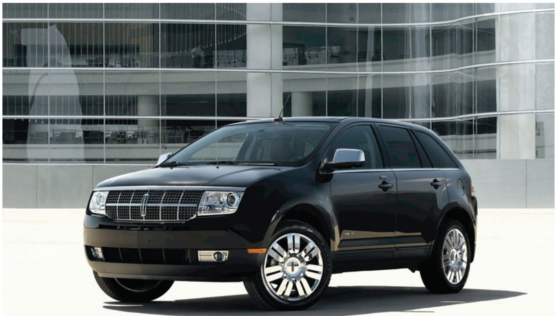
VEHICLES OF DIFFERENT SIZES, HEIGHTS AND WEIGHTS SHARE THE CD3 PLATFORM FIRST USED ON THE MAZDA6 FROM 2002. CLOCKWISE FROM ABOVE: LINCOLN MKX CROSSOVER, FORD FUSION SEDAN, AND SECOND-GENERATION MAZDA6 ESTATE
