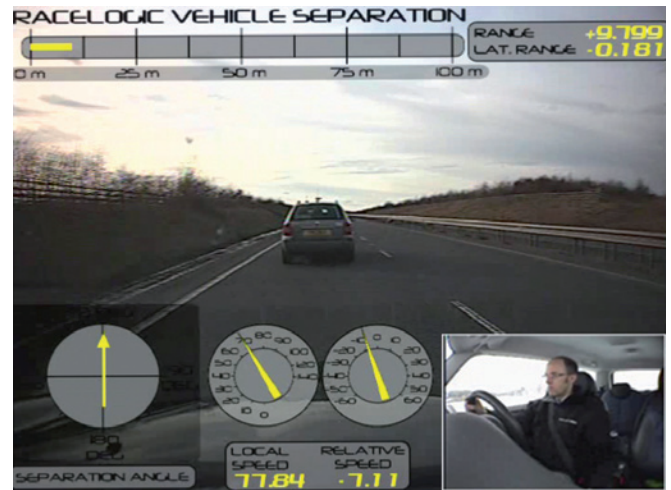
ABOVE AND BOTTOM OF PAGE: OVERTAKING WITH RACELOGIC'S VEHICLE SEPARATION SYSTEM AND VIDEO VBOX. LEFT: DIAGRAM TO ILLUSTRATE THE EQUIPMENT USED AND VEHICLE POSITIONING
