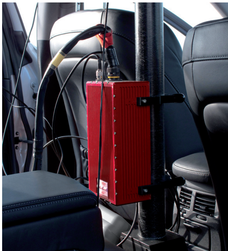
LEFT: RT3002 INERTIAL AND GPS NAVIGATION SYSTEM TO MEASURE VEHICLE'S MOTION, POSITION AND ORIENTATION
