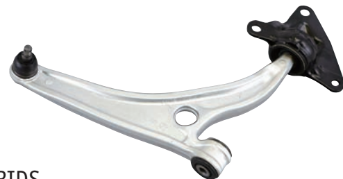
CR-Z FEATURES ALUMINUM FRONT SUSPENSION LINKS
