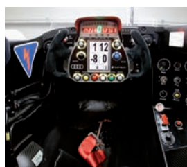
R15'S COCKPIT IS NARROWER THAN THE R10'S, RULING OUT BIGGER DRIVERS AND DEMANDING EXTRA DRIVER-CHANGE PRACTICE
