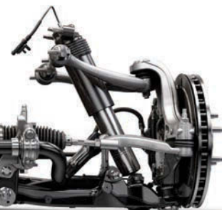
FRONT CORNER SHOWS DOUBLE-WISHBONE SUSPENSION SETUP
