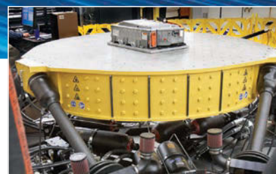
Vibration Testing: Hybrid/Electric Vehicle Battery Pack
