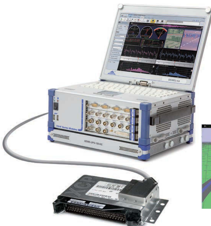
DEWE2 A4 WITH BATTERY OPTION AND XCP (LEFT) AND FUNCTIONAL SAFETY SCREEN (BELOW)
