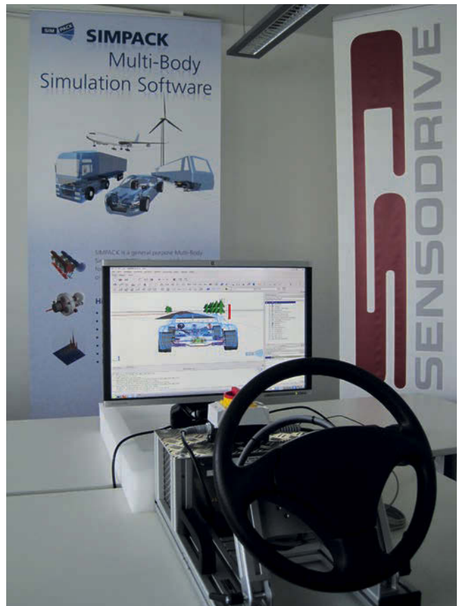
ABOVE: FIGURE 2: THE SIMPACK REALTIME DESKTOP DRIVING SIMULATOR USING A HIGH-PRECISION SENSODRIVE STEERING WHEEL
