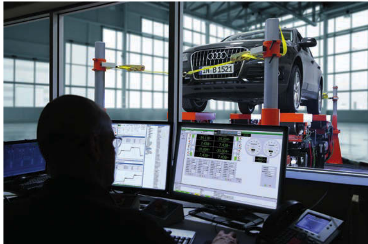
LEFT: LAB-BASED TUNING OF ACTIVE AND SEMI-ACTIVE SUSPENSIONS IS POSSIBLE, THANKS TO THE MOVING TIRES PROVIDING REAL VEHICLE FEEDBACK TO ECUS
