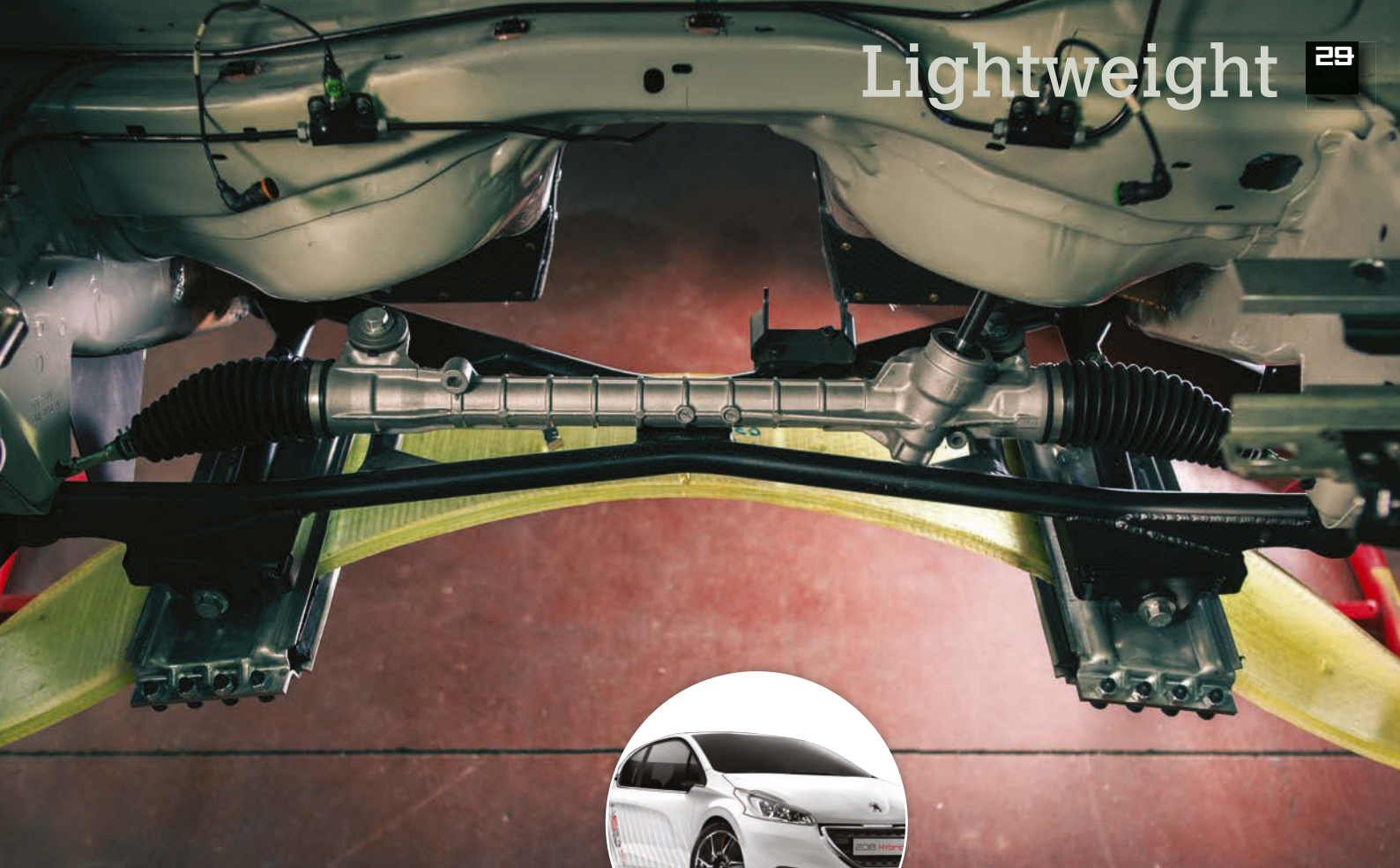
ABOVE: HUTCHINSON'S EPOXY MATRIX COMPOSITE TRANSVERSE LEAF SPRING SUSPENSION 'BLADE' ON THE PEUGEOT 208FE HYBRID (INSET)
