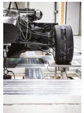
ABOVE: A FORMULA 3 CAR ON THE NEWLY OPENED RIG. THE WHEEL ACTUATORS OFFER 36KN OF DYNAMIC FORCE, THE AERO ACTUATORS 29KN
