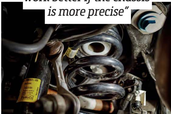
LEFT: Engineers for the Shelby GT350 found that having springs spin in different directions on each side of the car provided more rear-end stability. A counter-spun spring necessitated a new lower control arm design
