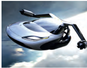
USA-based Terrafugia is developing Transition – a folding-wing, two-seat, roadable aircraft that drives like a typical car when on the ground
