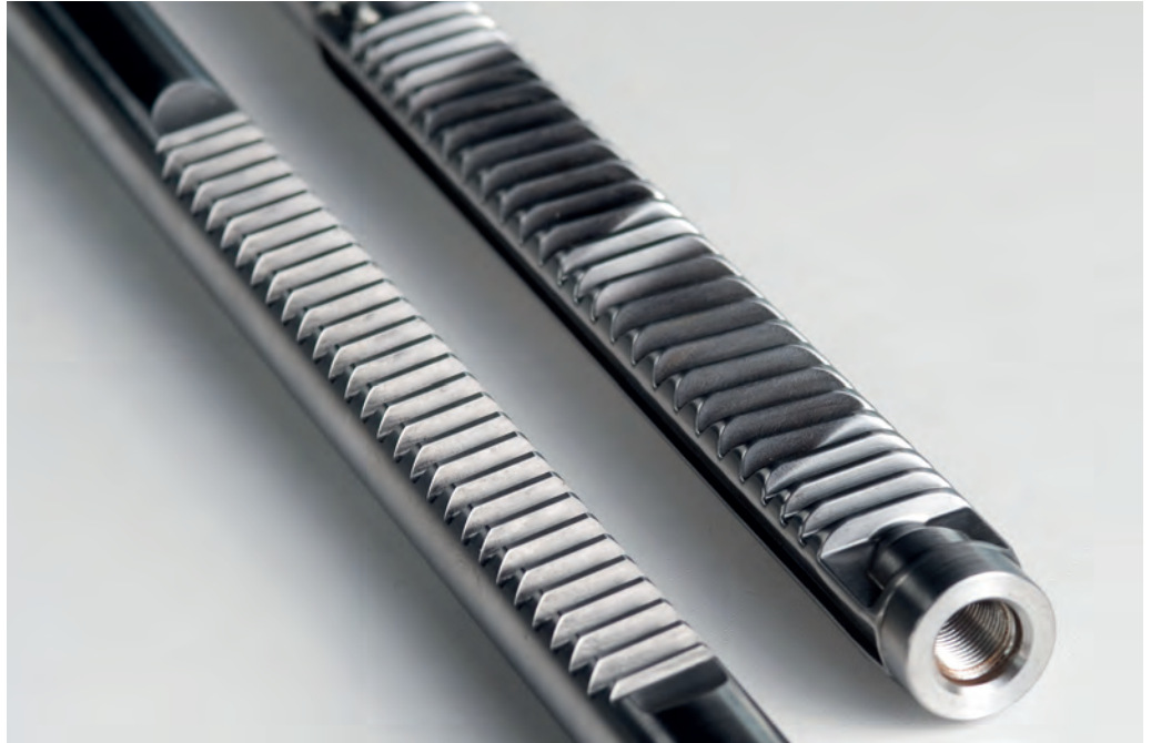
ABOVE: The precision warm-forged rack bar (on the right) has forged teeth, giving a wider, deeper cross-section
